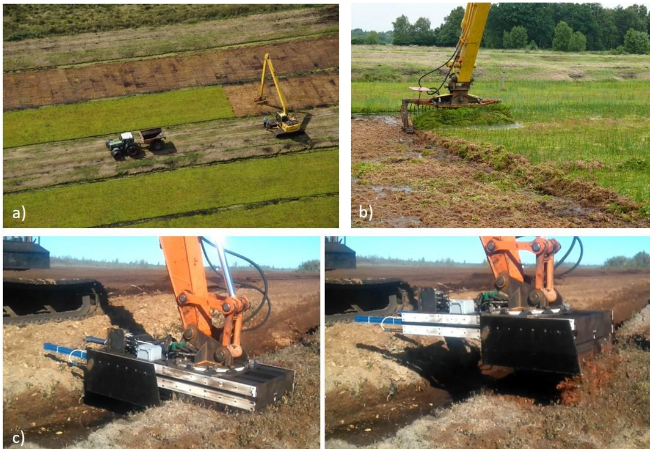
Figure 7. Harvesting techniques for Sphagnum farming using a) an excavator operating from a causeway, equipped with b) a mowing bucket or c) a modified excavator for block-cut peat extraction, which tests in Canada have shown can also harvest Sphagnum . Photos: a) Gerd Block, b) Sabine Wichmann and c) Benoit St-Hilaire).
