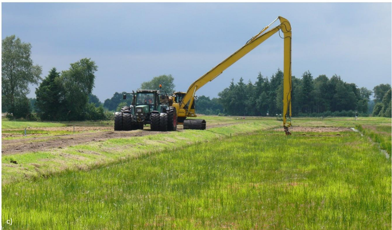
Figure 6. Weed management at the Rastede Sphagnum farming site using: a) brush cutter/trimmer; b) single-axle mower with cutter bar and triple tyres; c) excavator equipped with an extra-long arm and a mowing bucket, operating from a causeway. Photos: Sabine Wichmann.
