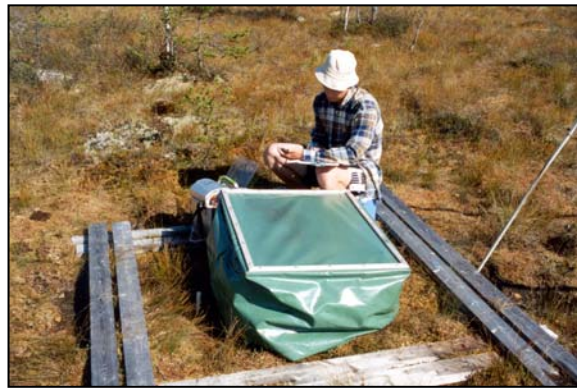
c) R_{TOT} measured with the chamber covered with an opaque plastic lid.
